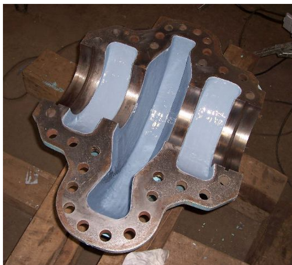
Coated housing improves the efficiency of the pump.
