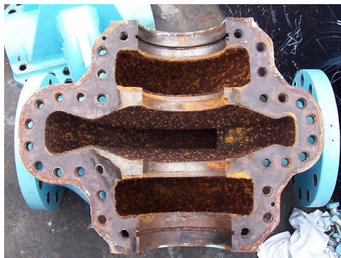
Split casing pump housing is corroded and inefficient.
