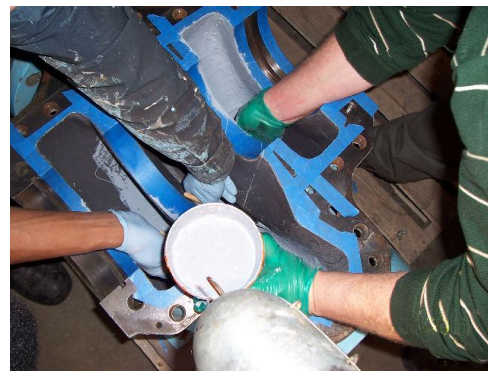
The housing is sandblasted and painted with polymeric coating.
