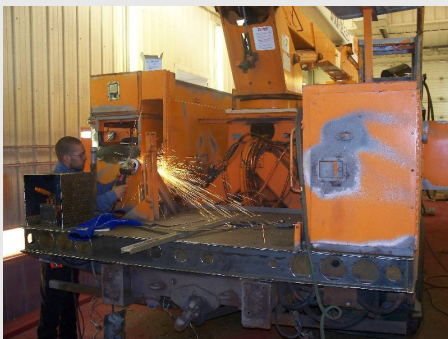
Fabricating parts for an electric boom truck.
